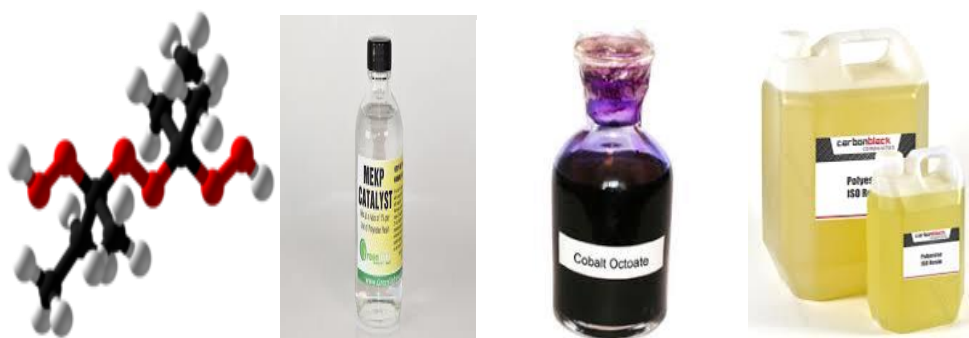
Fig: MEKP Structure, catalyst, cobalt and resin
