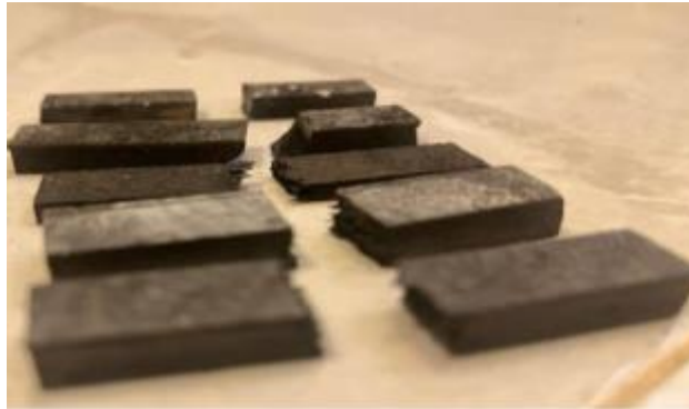
Figure 7: Specimens After Impact Tested of Epoxy fiber glass with Different weight Fraction of Nanoparticles
