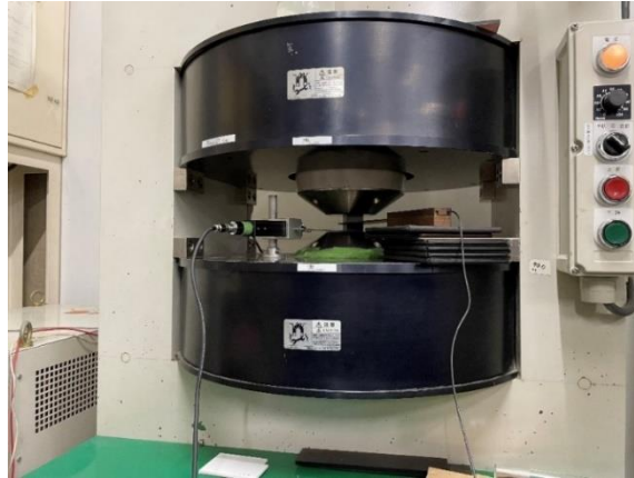
Figure 5 Experimental apparatus for magnetic properties measurements. BH analyzer (BH-1000H, Denshijiki Industry Co., Ltd.)
