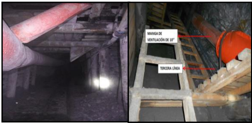
Picture 8. Ventilation with sleeve and third line in chimney.
