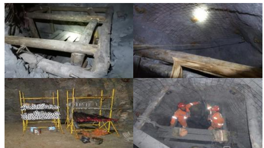
Picture 11. Supporting with over frames and mesh plus Split set in Chimney.
