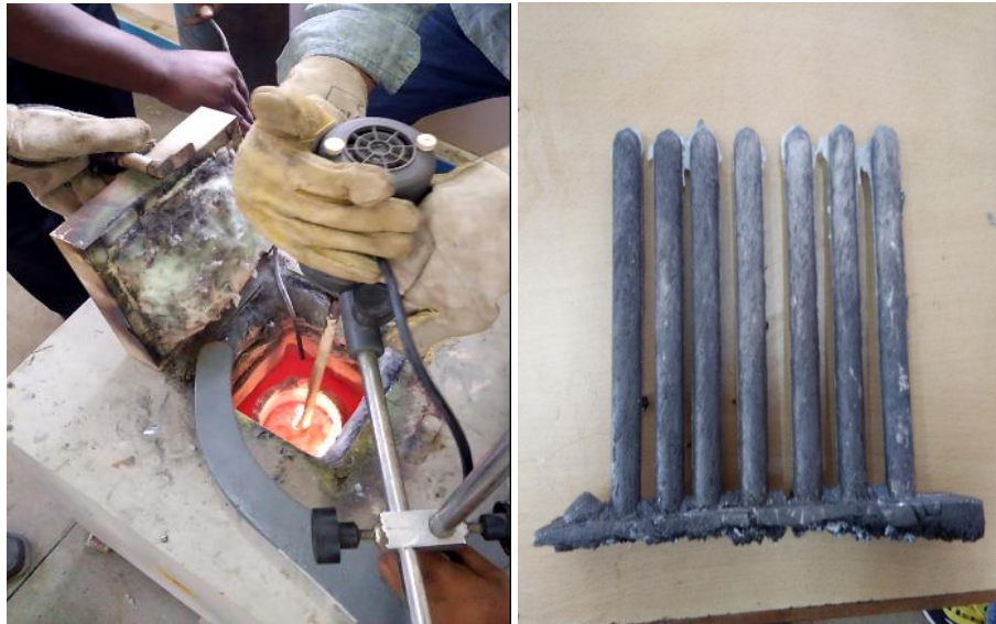
Figure 1. Stirring casting set up and composite fingers
