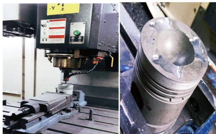
Fig 3.2.1 Photographs taken while making grooves on piston crown
