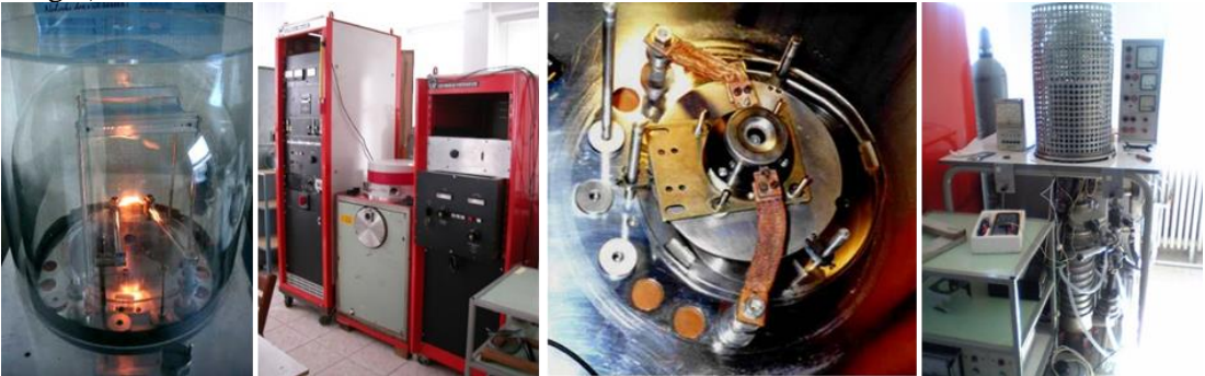
Figure 20. Physical vapor deposition device by heating the whole of the evaporating alloy in a tantalum crucible (left and left – center). Electron beam physical vapor deposition device (center-right and right).
