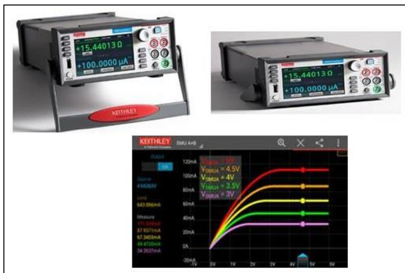
Fig:2. Photographical image of J-V analyzer (Keithley2450)
