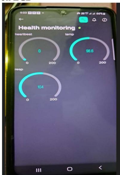
Figure 12. Increased Respiratory Level sent to Blink App using Iot Cloud Server
