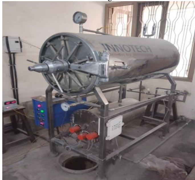
Fig 3 Steam Chamber Curing
