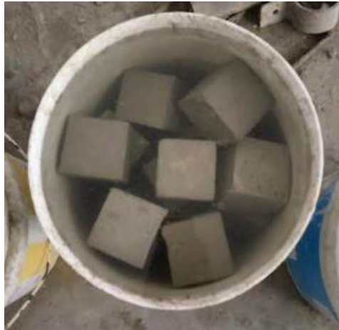
Fig 6 shows the Water Curing.
