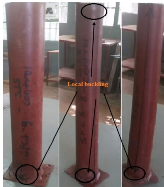
Fig. 4 Failure mode of unfilled steel tubes
