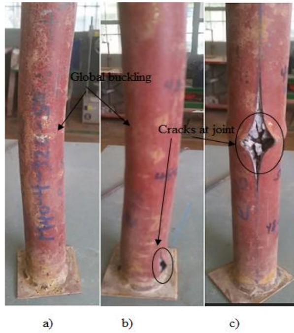
a) Global buckling b) Global buckling and cracking at bottom c) Local buckling and cracking at the middle Fig. 5 Different failure modes of TCSCFST
