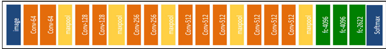
Fig. 3: VGG-Face model architecture
