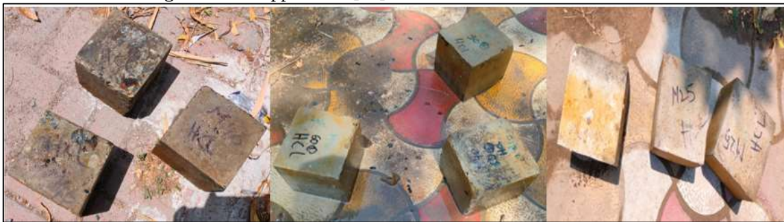
Figure 15. Physical appearance of M25, M40 and M70 grades GC samples after exposed to 5% HCl
