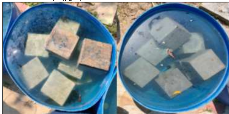
Figure 5. Cubes kept in water for water absorption test
