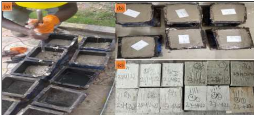
Figure 2. (a) Casting of cubes (b) Casted Cubes (c) Cubes kept for ambient curing
