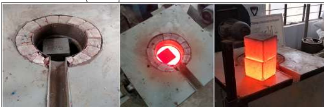
Figure 8. Tilting furnace and appearance of heated specimens
