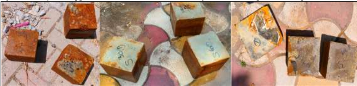
Figure 16. Physical appearance of M25, M40 and M70 grades GC samples after exposed to 5% H 2 SO 4
