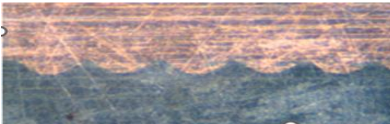
Fig.3. Bonding zone of the explosively welded NbTi (superconductor) sheet and copper sheet
