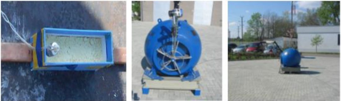
Fig. 6. Welding in the explosive chamber
