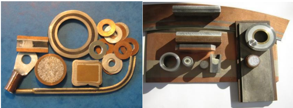
Fig. 1. More components materials prepared by explosive welding
