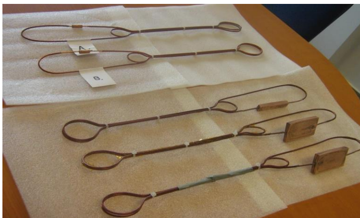
Fig.11. Explosively spliced superconductor test loops
