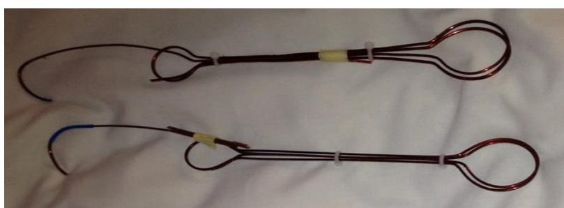
Fig.9. 1,39 m long cable samples for preparation of splice joint with copper sleeves
