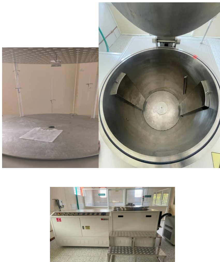
Fig.5 Coating of parylene on nafion 117 on 800 liters parylene deposition system of SCH coating solutions PVT ltd [17].
