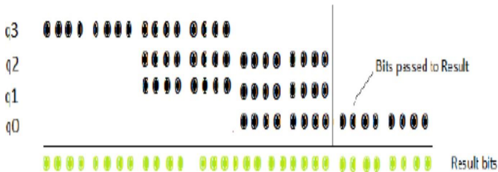
Figure 10: Addition of partial products in 16-bit Vedic multiplier
