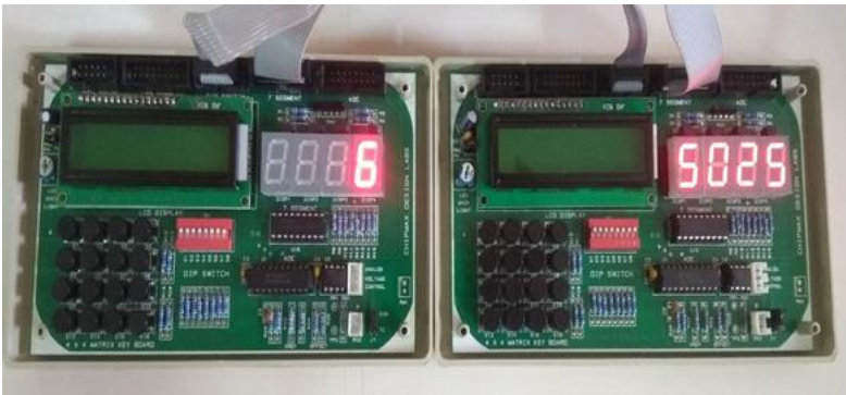
Figure 16. FPGA implementation of a 8-bit Vedic multiplier
