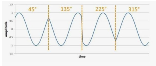
Figure 7 – Quadrature Modulation Diagram
