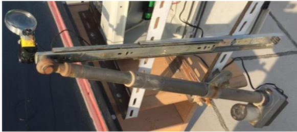
Fig. 3. Movement Part Mechanism (Axial & Rotation DC Motor)
