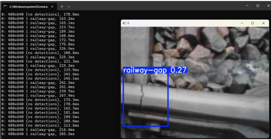
Fig 2: Railway Crack Detection using YOLOv7
