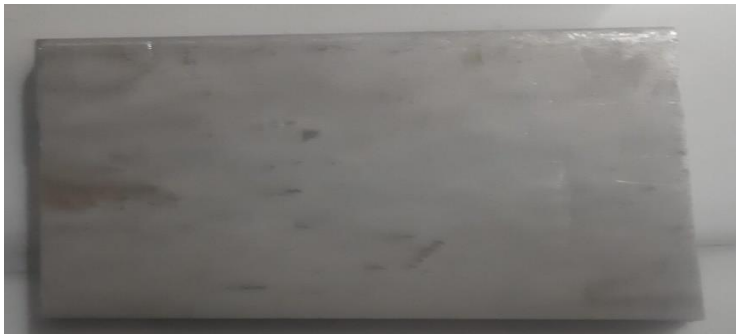
Figure 4: Stainless steel 316 workpiece material with size 150*100*10mm
