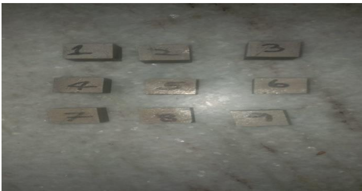
Figure 5: Stainless Steel 316 workpiece after machining
