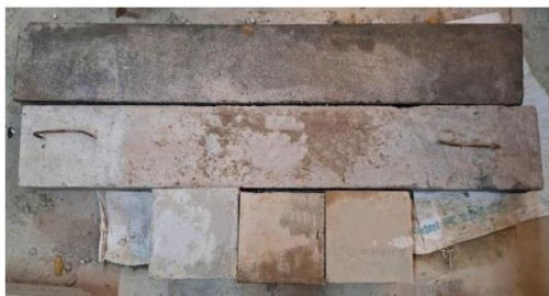
Fig-1 Solid beams with Cubes of M25 Grade
