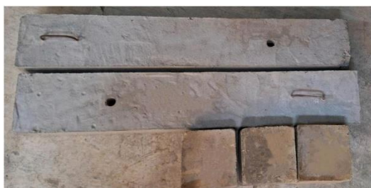
Fig-3 Solid beams with Cubes of M25 Grade
