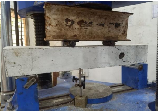
Fig-8 Testing on O-40 beam
