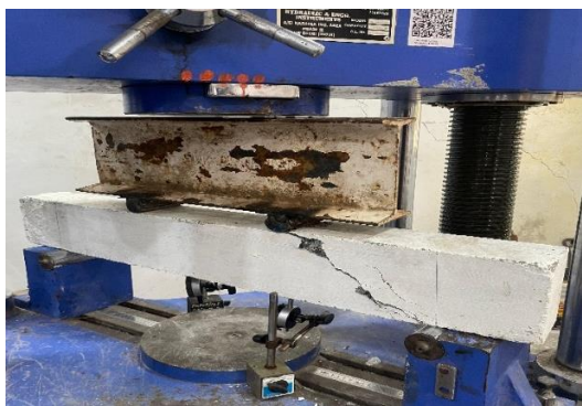
Fig-5 Testing on Controlled beam
