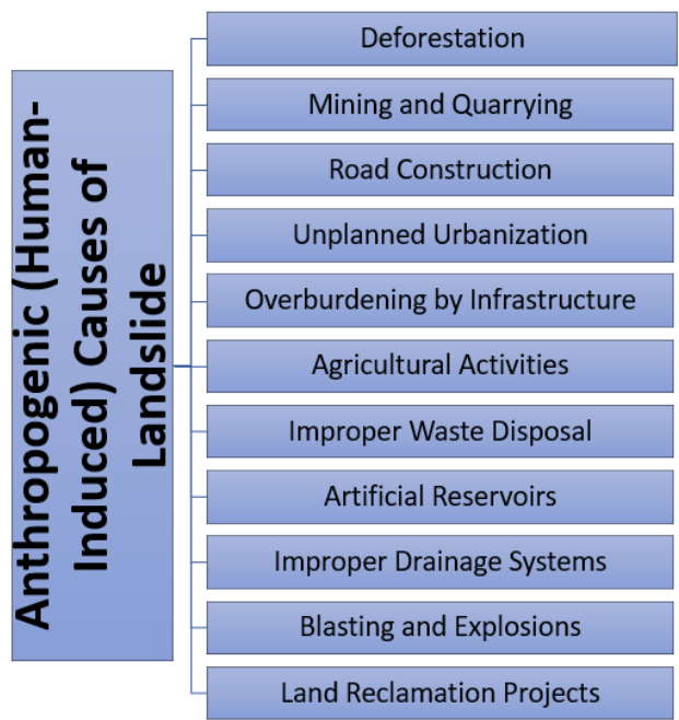
Fig. 2. Anthropogenic (Human-Induced) Causes of Landslide
