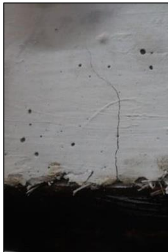
Figure 10 Flexural failure for specimen
