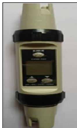
Fig 6 TDS, PH and Temp Meter for checking hardness and acidity of water
