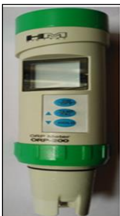
Fig 5 ORP Meter for checking the oxidation capacity of filtered water
