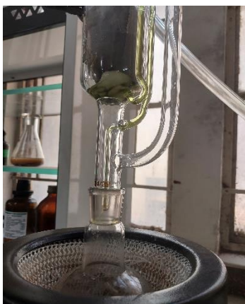
Figure 1: Extraction process of Guava leaves Powder
