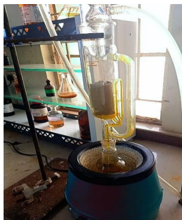
Figure 2: Extraction process of Turmeric
