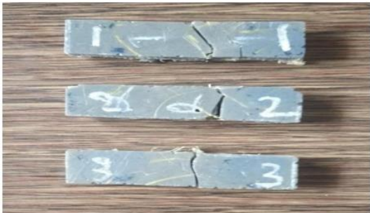
Figure 3.15: Broken specimens after impact test
