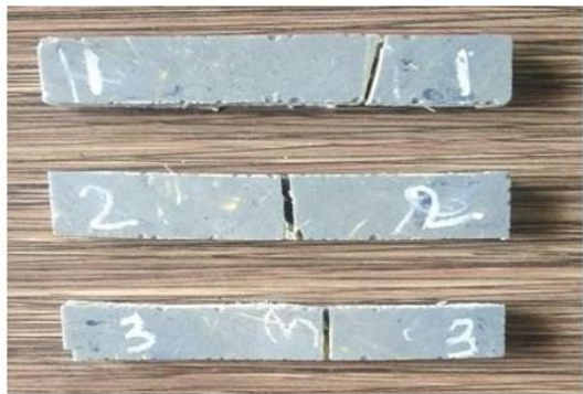
Figure 3.13: Broken specimens after flexural test
