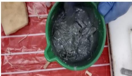
Figure 3.8: Final mixture of the composite material
