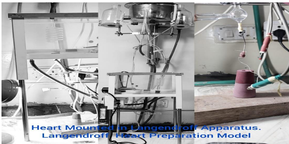
Fig.1 Langendorff Heart Preparation (Heart mounted in Langendorff Apparatus both global and regional ischemia can be studied using this model).
