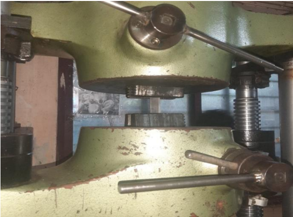
Fig 10 Compression Testing Machine Setup for Material Strength Analysis
