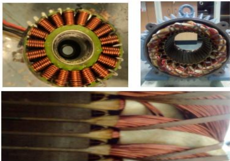
Figure. 5. Physical geometry of PM-type synchronous motor available in laboratory
