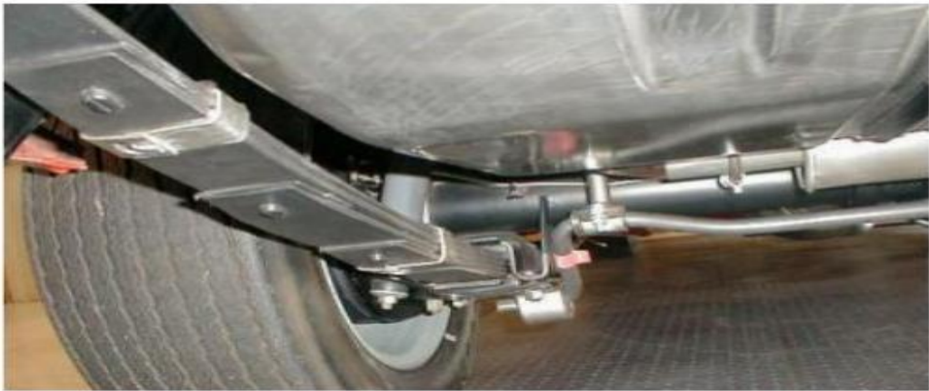
Figure 2: A Traditional Leaf Spring Arrangement.
