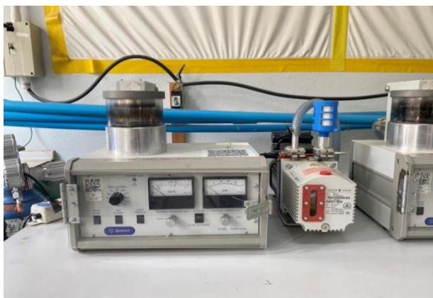
Figure 2. Sputter coater machine for Pd depositing process, Quorum Tech SC7620.
