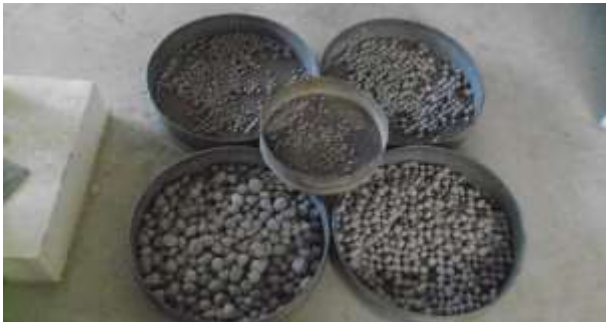
Figure 3: Collection of Fly Ash Aggregates from Mixer
