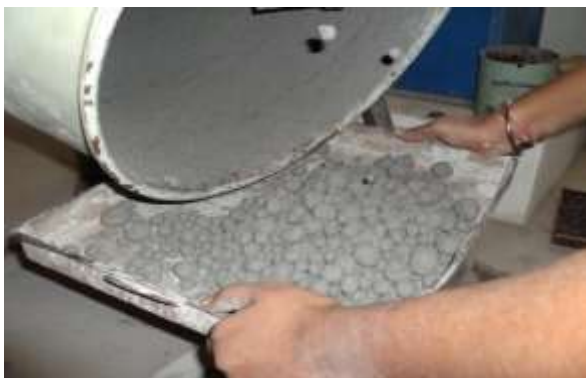
Figure 2: Collection of Fly Ash Aggregates from Mixer
