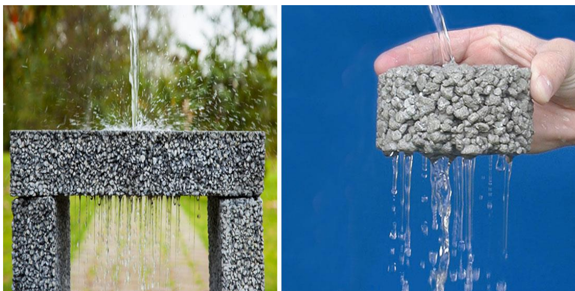
Figure 1: Hydraulic Conductivity and Water Retention Capacity of Permeable Concrete
