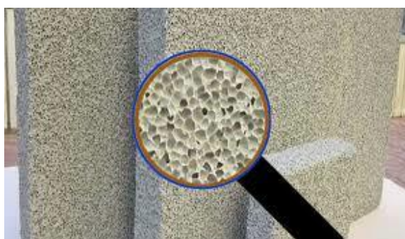
Figure 2: Microscopic Section of Sponge Concrete
