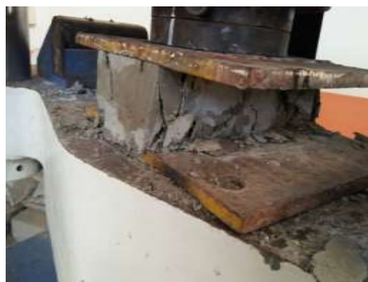
Figure 5. Compression strength test
