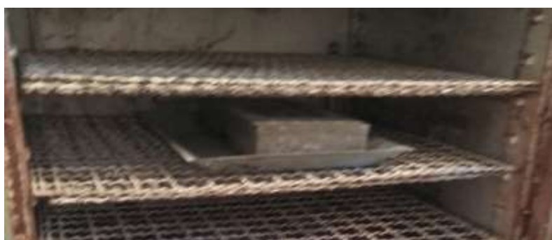
Figure 6. Brick exposed to high temp
