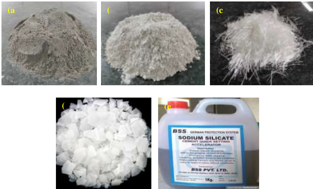
Figure 1. (a) Fly ash, (b) GGBS, (c) glass fiber (d) SH flakes and (e) SS
