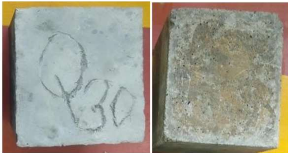
Figure 7. Cubes Before and After Dipping in Diluted HCl
