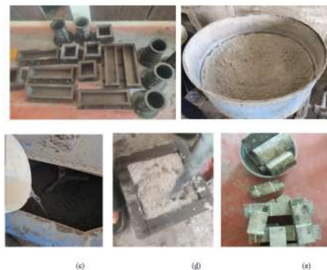
Figure 3. Mixing and Casting of Specimen
