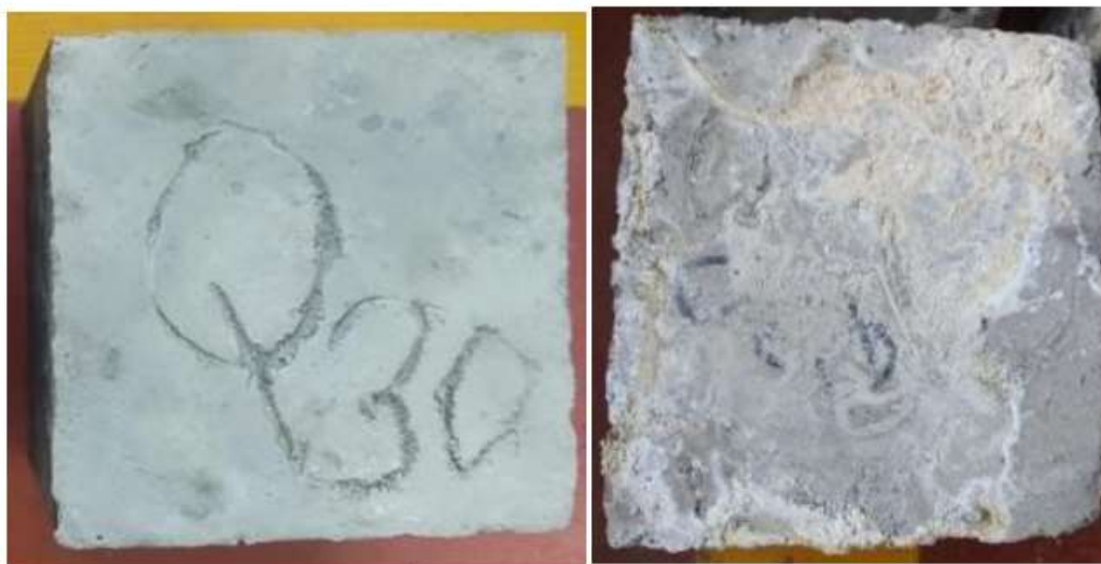
Figure 8. Cubes before and after dipping in diluted H 2 SO 4
