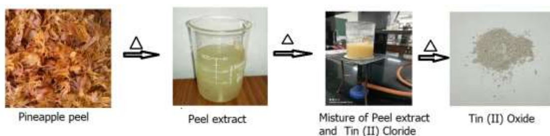
Fig. 1 Schematic representation of Synthesis of Tin (II) oxide nanoparticles using pineapple peel
