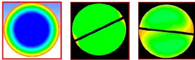
Figure. 19 Temperature contours in (K) for plain tubes, V-cut tubes, and alternate axis tape with ( TR = 4 ) and ( Re = 2002 ) at places along the test section with a ( Z = 50 cm) are shown
