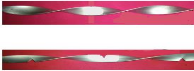
Figure.2 standard twisted tape and a V-cut twisted ratio inserts
