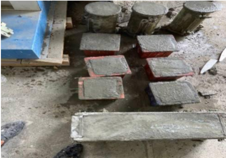
Figure 1. Casting of cylinders, cubes & prisms
