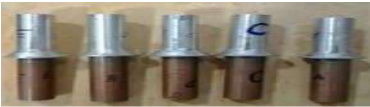
Fig 4. Aluminium+ Copper welding
