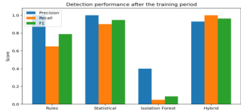
Figure 3. Precision, recall, and F1 by detector.
