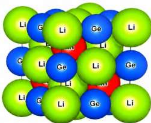
Figure 1. Representative lattice structure of the \text{Li}_2\text{MnGe} alloy.
