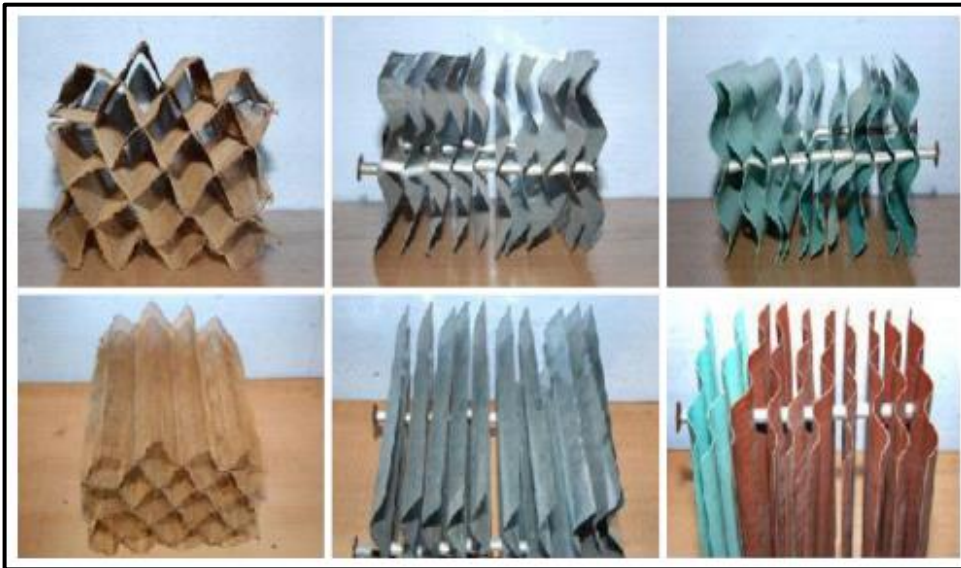
Figure 6: Packing materials for cooling towers (EWM, GI, PVC)[55]
