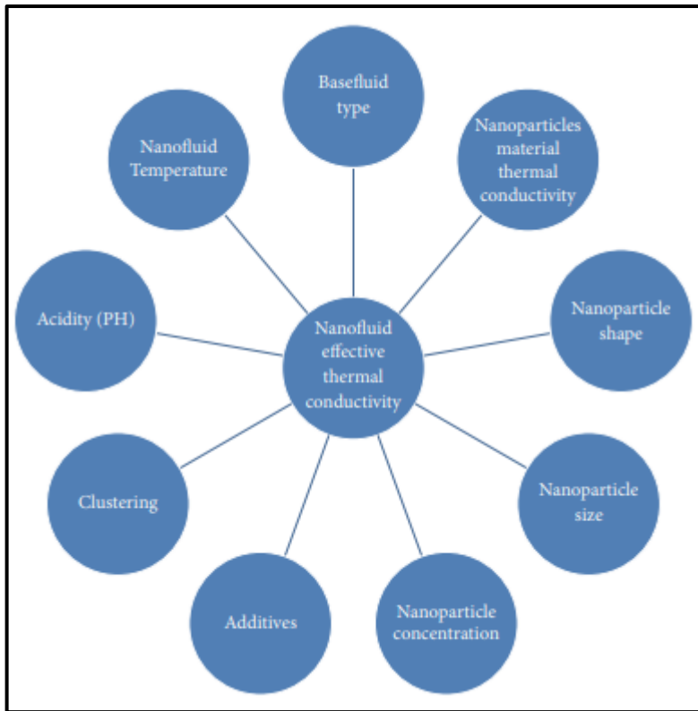
Figure 10: Nanofluid thermal conductivity is affected by the aforementioned factors [62]
