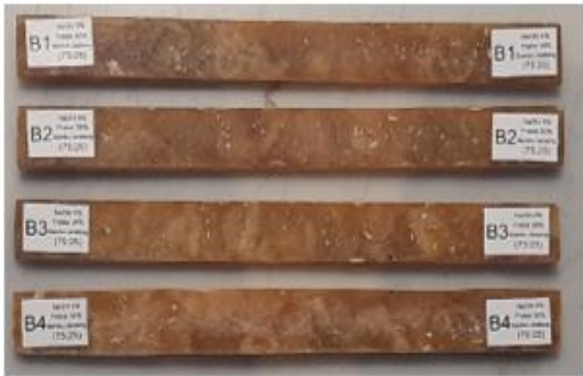
Fig. 2. Example of a tensile testing specimen
