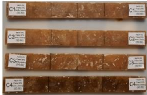
Fig. 3. Examples of flexure testing specimens
