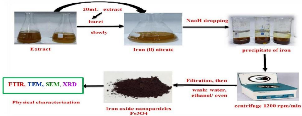
Figure 2: Schematic diagram of green synthesis of \text{Fe}_3\text{O}_4 -NPs of C. Spinosa
