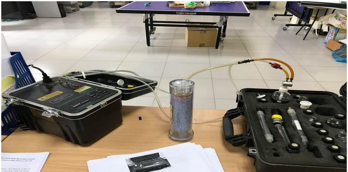
Figure 2: RAD7 machine and tool set RAD - H_2O
