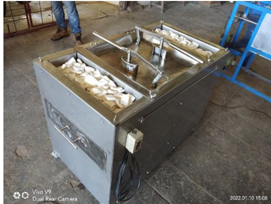
Figure 3. Photo of the coconut meat chipper
