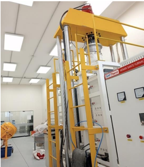
Figure 2. Prototype equipment for the mechanical, thermomechanical and controlled atmosphere evaluation of materials of standardized size
