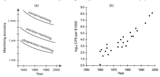
Figure 1. (a) On the left, the evolution of machining accuracy (after N. Taniguchi). (b) On the right, the evolution of the number of calculations per second (CPS) obtainable per \$1000 of digital computer, starting with the IBM 1620 and ending with the Pentium II PC [20]. Note that the vertical scale is logarithmic in both cases. In its original form [23], Moore's Law asserted that the number of components per chip doubles each year.
