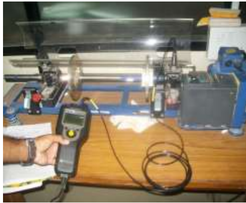
Figure 1. experimental setup of Rotating Disk Assembly with Dual Bearings and Motor Drive
